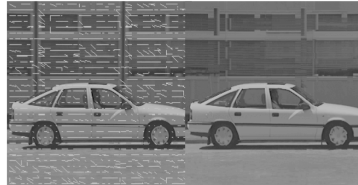
Frame with motion vectors Motion-compensated prediction
