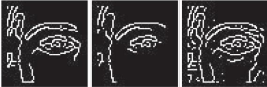
Hysteresis thresholding, upper level = 40, lower level = 10
