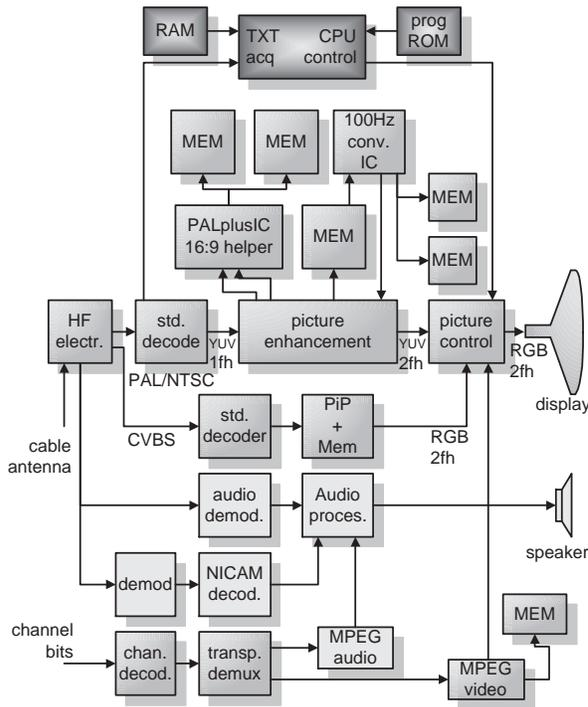
Fig. 1. The HW architecture of a conventional high-end TV set.
