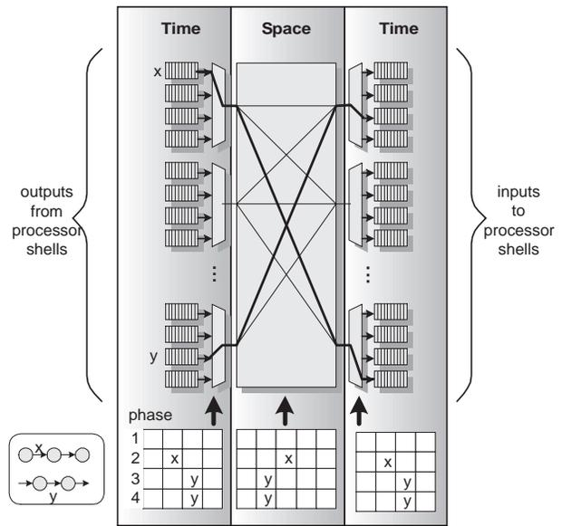
Fig. 8. A Time-Space-Time (TST) network, ensuring a guaranteed bandwidth for hard real-time tasks.
