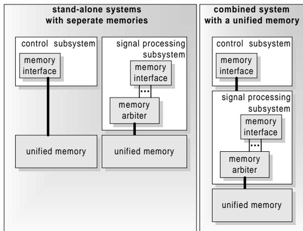
Fig. 10. Stand-alone systems and a combined system with unified memory.
