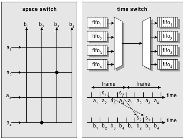
Fig. 7. A space switch (left) and a time switch (right).
