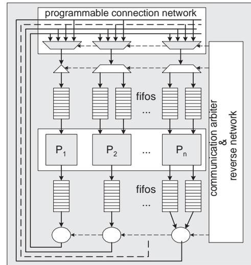
Fig. 5. The architecture of the signal processing subsystem.
