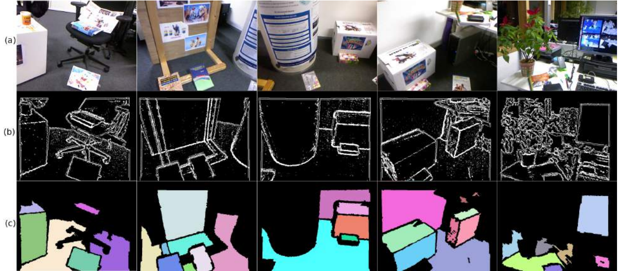
Fig 5 Five examples of datasets containing various types of 3D edges and the corresponding outcomes: (a) color images of each scene, (b) extracted 3D edges, and (c) planar surfaces (Note that the merging and size-validation phases have not been incorporated in the visual results).
