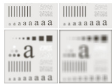
FIGURE 3.33 (a) Original image, of size 500 \times 500 pixels. (b)–(f) Results of smoothing with square averaging filter masks of sizes m = 3, 5, 9, 15, and 35 , respectively. The black squares at the top are of sizes 3, 5, 9, 15, 25, 35, 45, and 55 pixels, respectively; their borders are 25 pixels apart. The letters at the bottom range in size from 10 to 24 points, in increments of 2 points; the large letter at the top is 60 points. The vertical bars are 5 pixels wide and 100 pixels high; their separation is 20 pixels. The diameter of the circles is 25 pixels, and their borders are 15 pixels apart; their intensity levels range from 0% to 100% black in increments of 20%. The background of the image is 10% black. The noisy rectangles are of size 50 \times 120 pixels.
