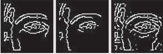
Hysteresis thresholding, upper level = 40, lower level = 10
