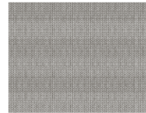
FIGURE 5.17 Noise pattern of the image in Fig. 5.16(a) obtained by bandpass filtering.
