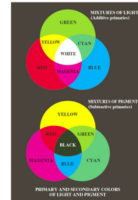
FIGURE 6.4 Primary and secondary colors of light and pigments. (Courtesy of the General Electric Co., Lamp Business Division.)
